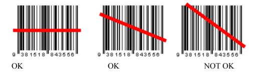
It is important that the bean goes across ALL the lines – in the examples above, the left and middle scans would be OK, the right hand one would not work. Also, do not hold the barcode too close to the scanner – about 100mm (4") is ideal.
